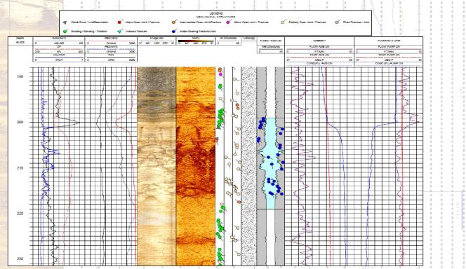
The results of the study showed that: 1) water bearing fractures were a small percentage of the total number of fractures observed in the borehole; 2) the water bearing fractures were present among all the major geologic units; 3) the water bearing fractures displayed high hydraulic conductivity; and 4) the PFAS contamination appeared widely dispersed vertically, as the deepest water bearing zones (at 300 feet) were contaminated.
